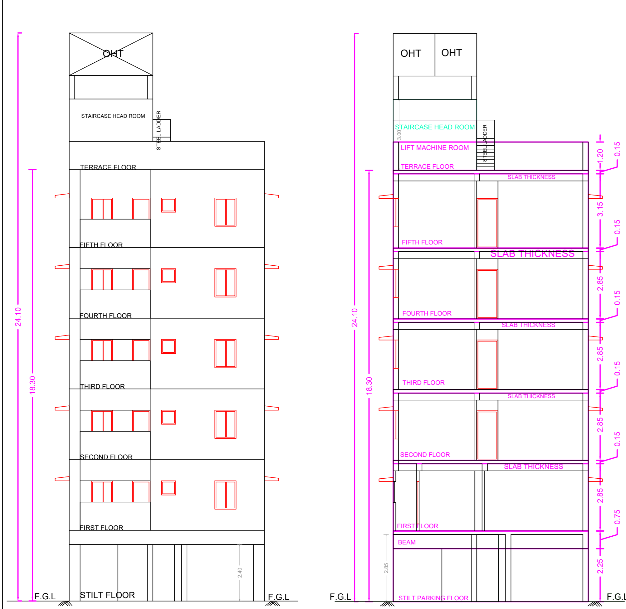
ELEVATION SECTION ON A-A
