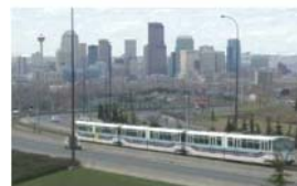
Calgary - Metro on Grade in Centre of Expressway
